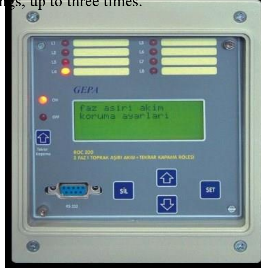
Figure 1. Front panel view of ROC 200C 3 phase + 1 ground overcurrent protection relay
